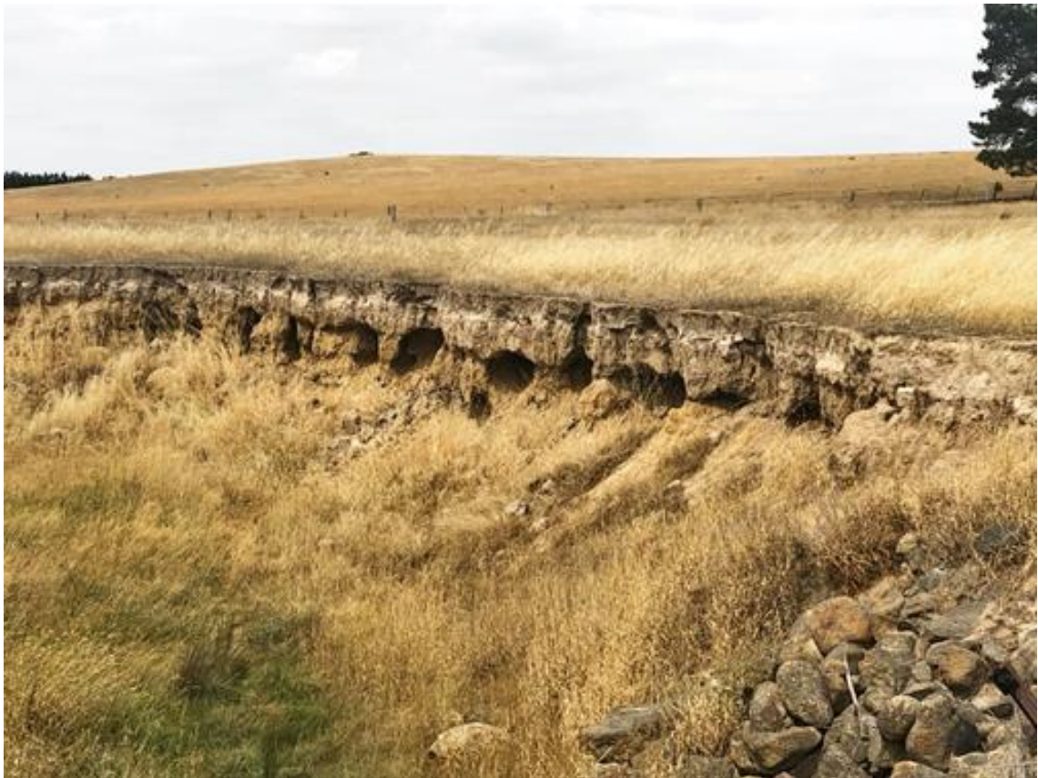
Figure 6-2 Example of eroded dispersive soils near the town of Beveridge (GHD, 2020)
